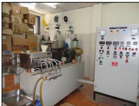
Fig 1. Twin screw extruder (Department of fish processing, Central Institute of Fisheries Education, Mumbai)
